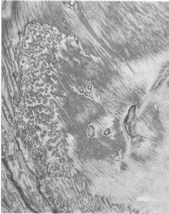
FIGURE 5 Fracture surface micrograph obtained with reflected green light. The low-molecular-weight polystyrene layer between the poly(methyl methacrylate) plates had a thickness of approximately 0.1\ \mu\text{m} . The white bar represents 20\ \mu\text{m} .
